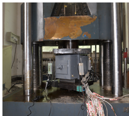
图14 模块化组合结构连接节点剪切性能试验 Fig. 14 Shear performance test of connecting nodes in modular composite structures
