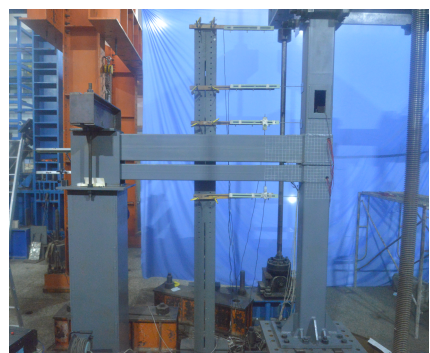
图12 模块化钢结构高强度螺杆连接节点框架试验 Fig. 12 Modular steel structure high-strength bolted Joint frame test
